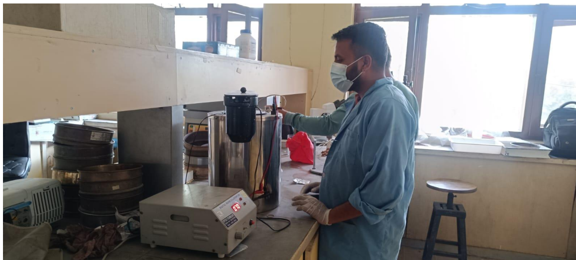
Photo 1: Measuring the calorific value of the organic waste samples brought from the field at CDES laboratory
